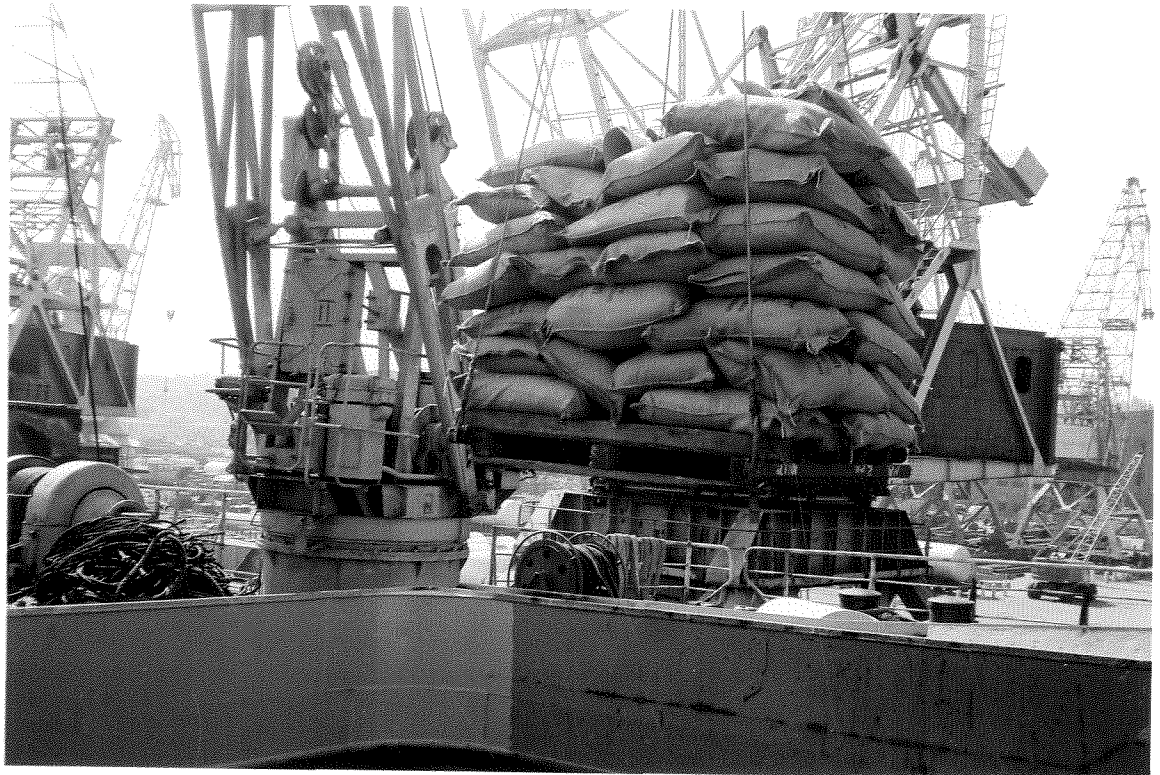
A slingload clearly too large to safely hoist.
